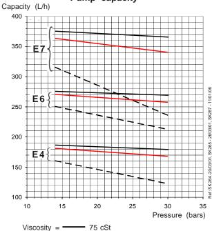
Viscosity = 75 cSt 20 cSt 5 cSt - Rated speed = 2850 rpm
